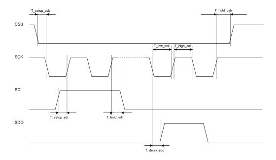
Figure 13: SPI timing diagram
