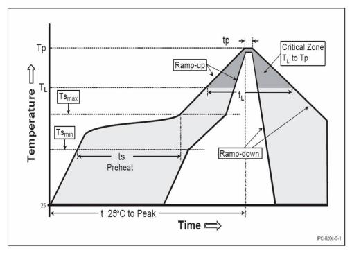
Figure 20: Soldering profile
