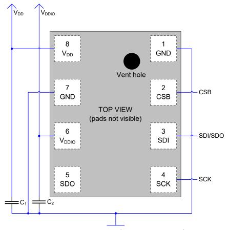
Figure 16: 3-wire SPI connection diagram (Pin1 marking indicated)
