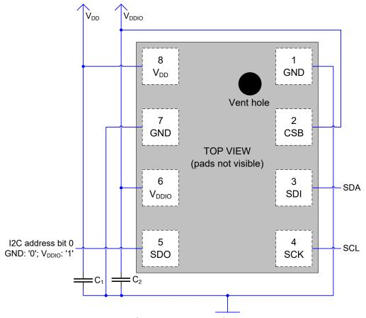
Figure 17: I2C connection diagram (Pin1 marking indicated)
