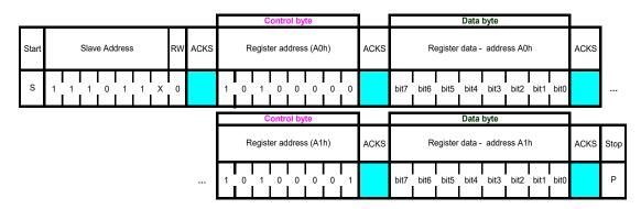
Figure 7: I2C multiple byte write (not auto-incremented)
