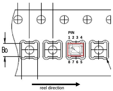
Figure 22: Orientation within tape
