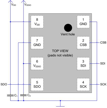
Figure 15: 4-wire SPI connection diagram (Pin1 marking indicated)
