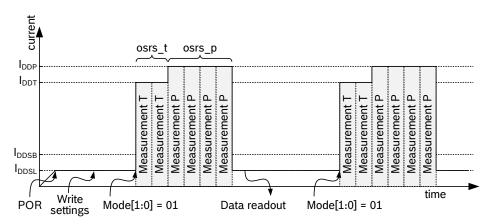
Figure 3: Forced mode timing diagram
