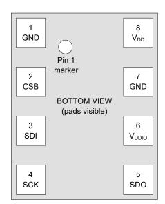
Figure 14: Pin-out top and bottom view
