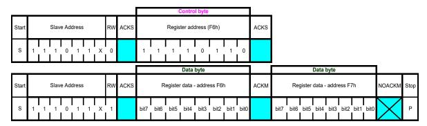
Figure 8: I2C multiple byte read
