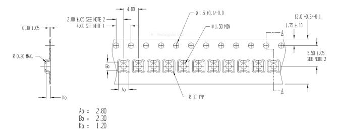
Figure 21: Tape and Reel dimensions
