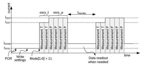
Figure 4: Normal mode timing diagram
