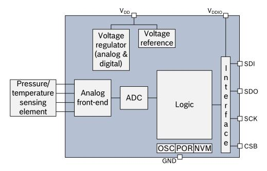
Figure 1: Block diagram of BMP280
