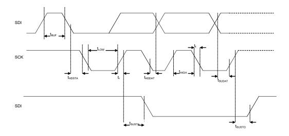
Figure 12: I<sup>2</sup>C timing diagram
