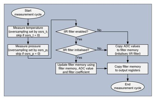
Figure 2: BMP280 measurement cycle
