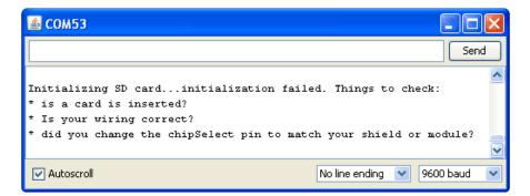
It couldn't even initialize the SD card. This can also happen if there's a soldering error or if the card is really damaged
