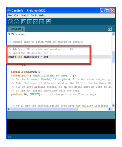
If you have the pre-rev B version of the Datalogger Shield, and you are using a Mega or Leonardo check here for now to adjust the pin setup ()
