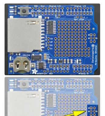
This is the "R3 compatible" Datalogger. Note that it has a smaller prototyping area and that there is a 2x3 SPI header spot on the right
